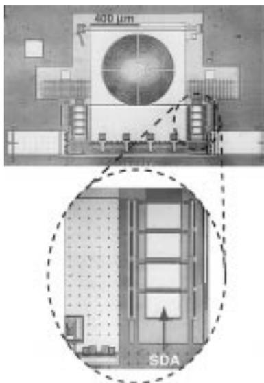
Fig. 4. The top-view photograph of the micro-Fresnel lens in the micro-XYZ stage integrated with eight scratch drive actuators (SDA) before assembly. The dimension of the lens is  $800\ \mu\text{m} \times 1020\ \mu\text{m}$ .
