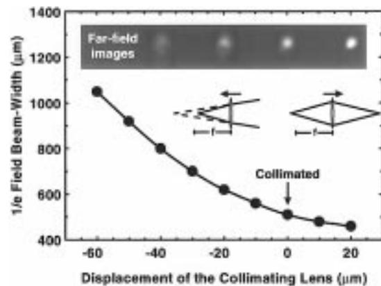
Fig. 3. Focal length adjustment by changing the position of the collimating lens along the optical path (Y-direction).
