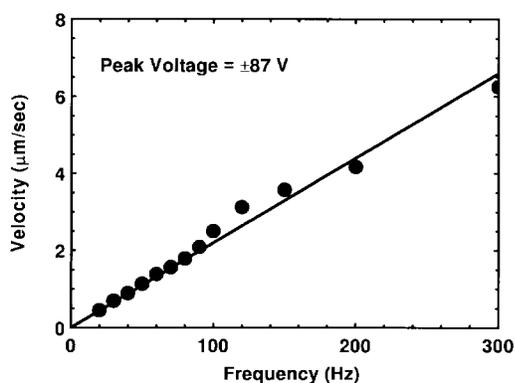
Fig. 5. The velocity of the assembled micro-Fresnel lens in the micro-XYZ stage versus the actuating frequency of the SDA.
