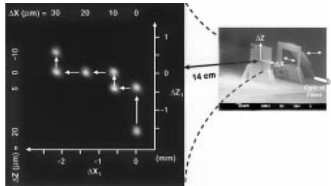
Fig. 2. Two-dimensional (X-Z plane) optical beam scanning by moving the lower and upper 45° mirrors of the micro-XYZ stage independently.
